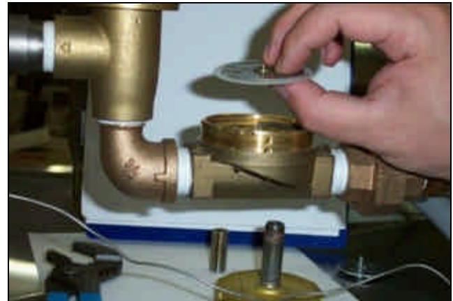
Removing the diaphragm
